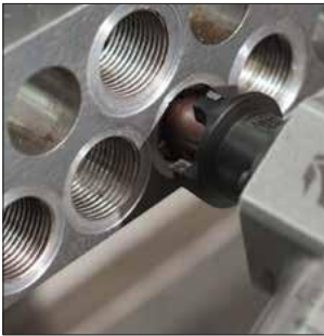
Safely re-machine gasket surfaces in seconds.
